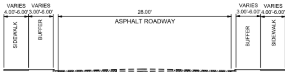
Figure 5: 7 th Street Existing Typical Section
